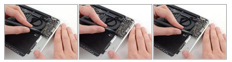
Use the tip of a spudger to carefully flip up the retaining flap on the microphone ribbon cable ZIF socket.
