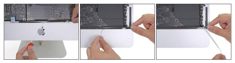
Peel away the white backing behind the strip to expose the remaining adhesive.
