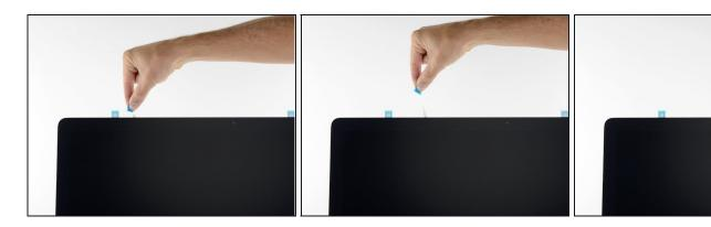
Remove one side of the protective film from the top left strip by pulling its tab straight up.
