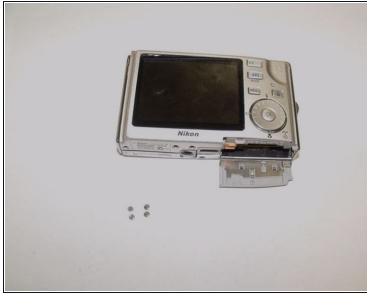
• Remove the four screws adjacent to the SD/battery opening using a Phillips #00 screwdriver.
