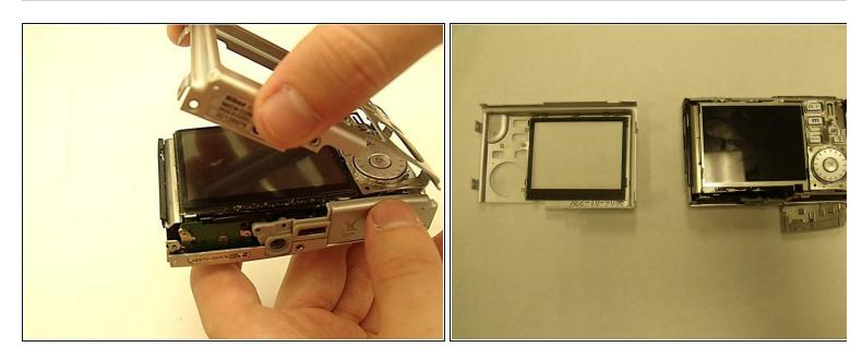
• Separate the back faceplate from the rest of the camera.
