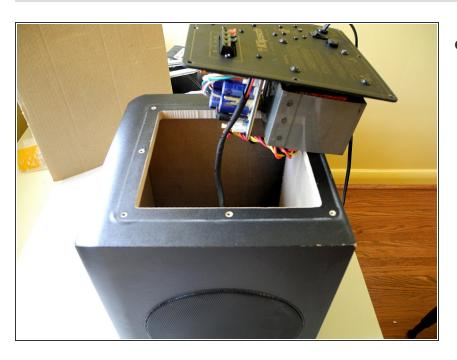
When you've finished removing all 8 amp screws, SLOWLY lift the amp assembly out of the sub enclosure. Be careful. The red and black speaker wires encased in black insulation that connect the amp to the speaker are a bit tight. Don't pull the speaker wires or you could damage something.
