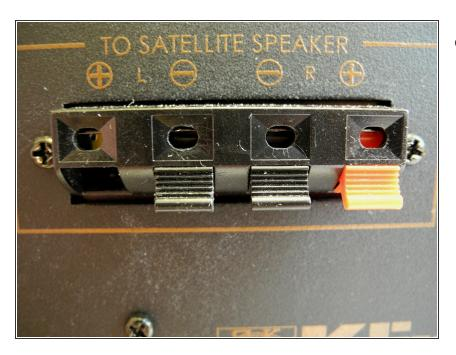
Now, carefully move the amp assembly and the wooden enclosure enough so that you can see the speaker terminals on the rear of the amp. Undo the two screws (on each side of the speaker terminals), and set them aside, noting where they came from.
