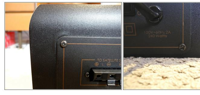
• Find the eight (8) screws around the periphery of the metal amp that fasten the amp to the wooden subwoofer enclosure. Notice that all 8 screws sit on top of, or at the intersection of the outermost gold lines. Undo these eight screws. DON'T undo any other screws at this time.
