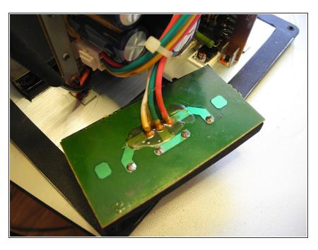
Now, gently and carefully put the amp assembly back down onto your work surface. Notice the green PCB (circuit board) there. That's the PCB for the speaker terminals, surrounded on one side by some foam insulation to prevent air leakage.
