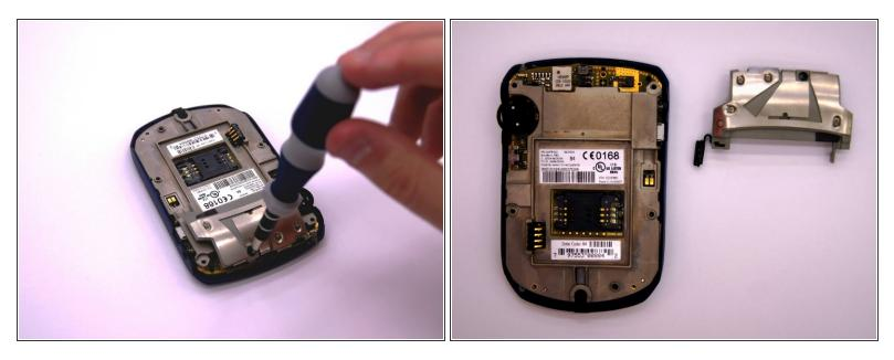
Using a Torx T6 screwdriver, remove the lone 1/8 inch screw that holds the upper metal bracket onto the larger metal bracket. Set aside the screw and the bracket.
