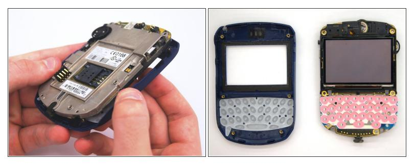
• Remove the front plastic case from the metal bracket.
