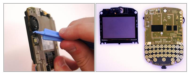
• Use the plastic opening tool to pry at the edge of the screen near the track-wheel.
