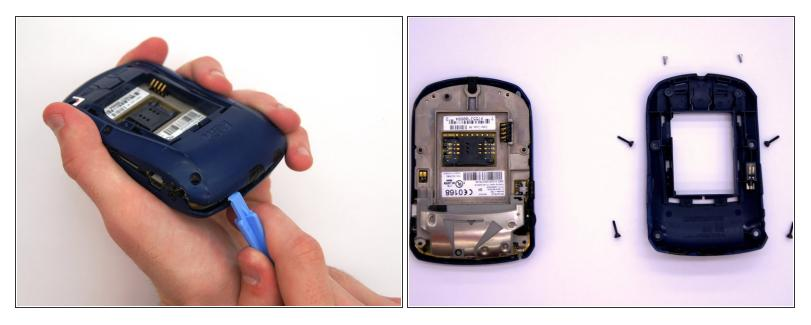
Use the plastic opening tool to pry the back case away from the front case.
