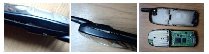
• Once the back cover is off, one can see the motherboard and a strange metal part on the top of the phone. This serves as an antenna booster, but also to protect the board.
