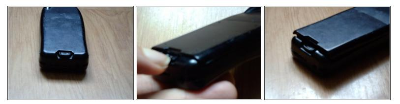
• The battery is removed easily. Just pull down the part from the back and the battery goes out.
