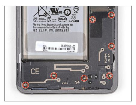
Remove the seven 4 mm Phillips screws securing the lower midframe to the phone.
