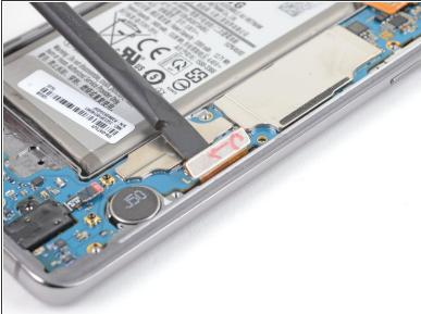
Use the flat edge of a spudger to pry up and disconnect the display connector from its motherboard socket.
