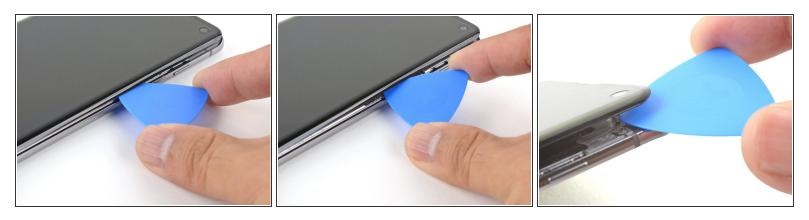
Use an opening pick to pry open and slice through any remaining adhesive.
