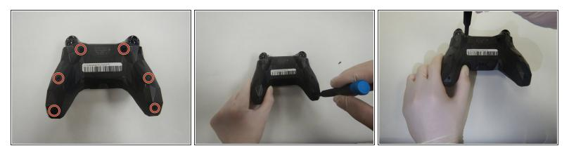
• Use a Torx TR6 screwdriver to remove the six 7mm screws from the back of the controller.
