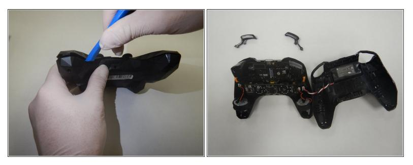
• Use a plastic opening tool to pry open the back frame of the controller.
