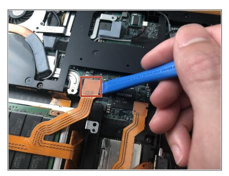
Use an opening tool to pry the uSATA ribbon cable connector up from its socket on the motherboard.
