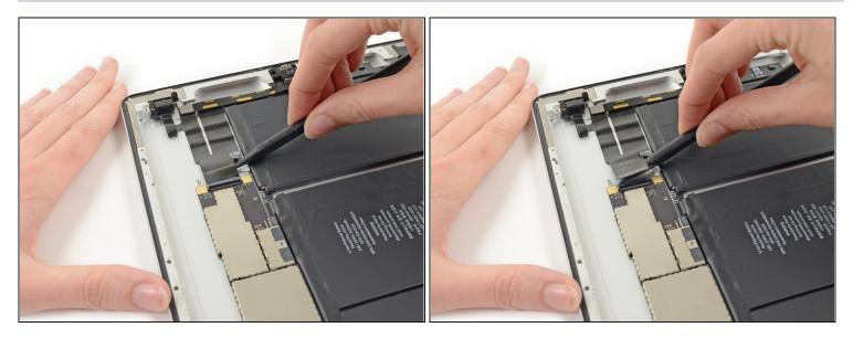
• Slide the tip of a spudger underneath the headphone jack/control board ribbon cable to disconnect it.
