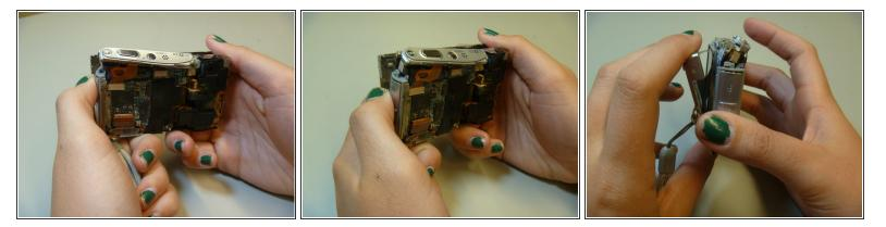
• Pull apart the inner hardware from the back case by prying on the left side.
