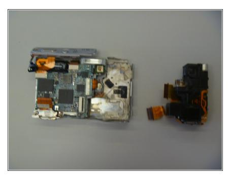
• The CCD module is now removed from the camera.
