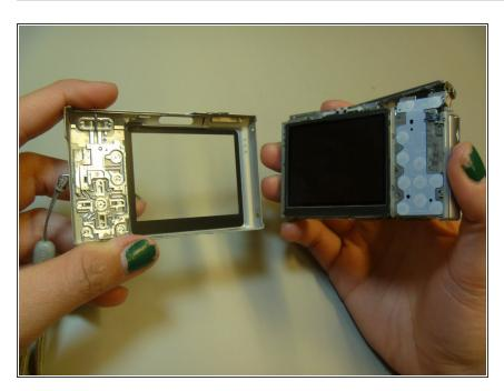
• The back cover is now removed from the internal hardware.
