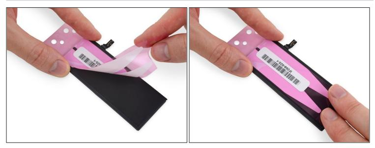
• Lay the strips down flat on the back of the battery.
