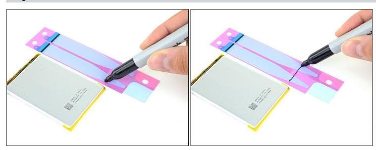
• Using a pen, mark a line on the stretch release adhesive just slightly above the bottom edge of the battery.
