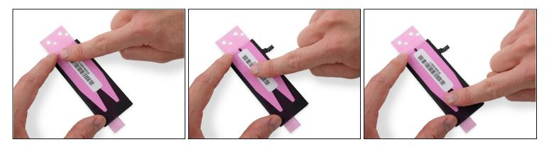
Use your fingers or a cloth to press the strips firmly into place along the back of the battery.
