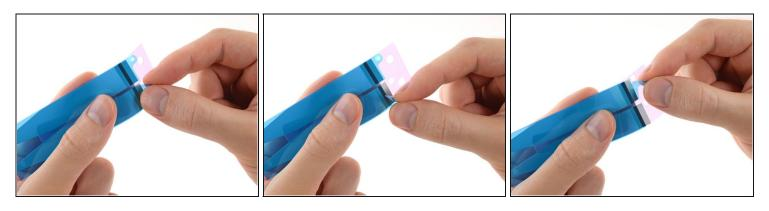
• Remove the small sections of blue film covering the flat ends of the adhesive strips. Don't remove the entire blue liner, just the small parts covering the pull tabs.
