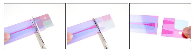
• Use a pair of sharp scissors or a razor blade to cut the stretch release adhesive tabs at the marked line.
