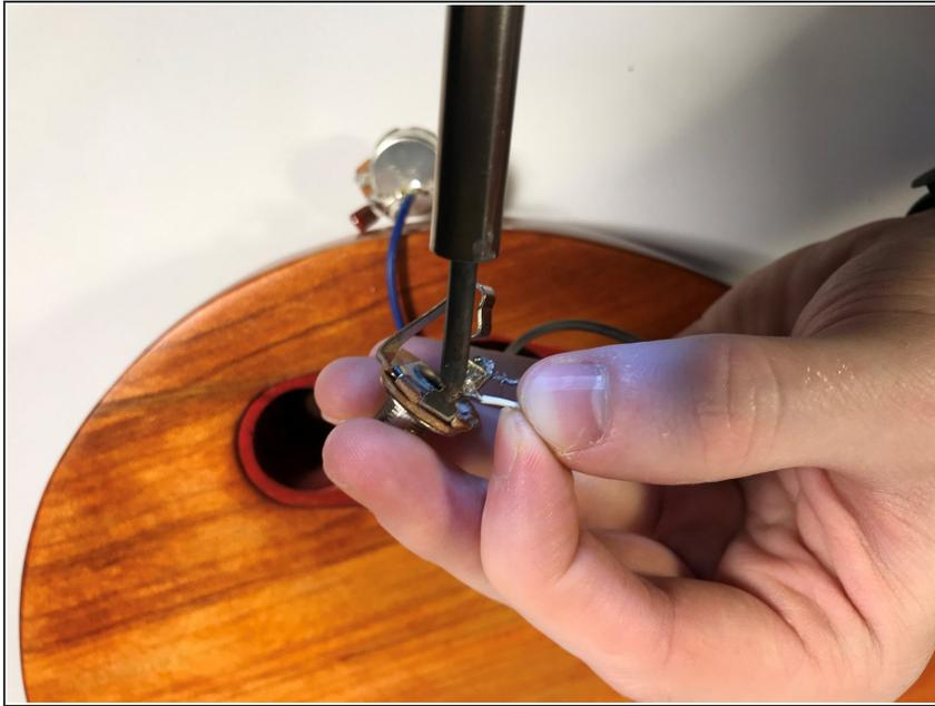
**⚠** The soldering iron is very hot. Avoid contact with skin, as well as the body of the instrument. When not in use, place it on a soldering iron stand.
