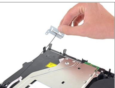
Remove the Wi-Fi antenna.
