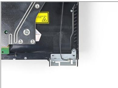
Remove the 9.7 mm Torx security screw securing the antenna.
