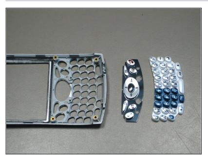
Remove the keypad for cleaning or replacing.
