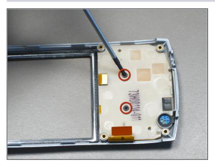
Unscrew the two 3.2 mm screws with a Phillips #00 screwdriver.
