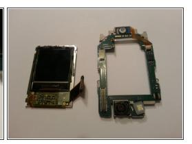
Remove the connector at the bottom left side of the logic board with the pictured orientation in mind.
