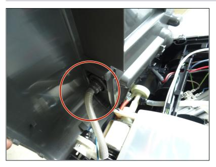
Pull off the silicone hose that leads to the water connection of the tank from the inside.
