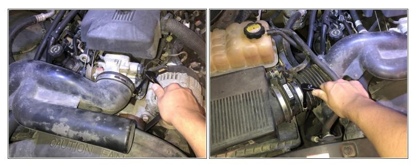
Loosen the hose clamps on the factory intake tube with an 8mm socket and remove the intake tube. One hose clamp will be located at the port of the intake manifold and one will be near the factory air box.
