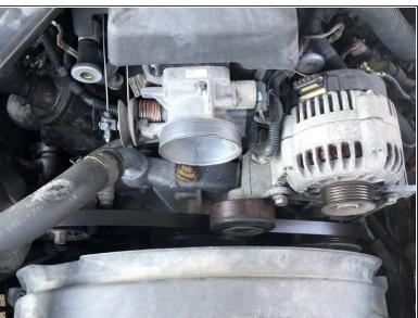
Using a 15mm socket on a half inch socket wrench, loosen the belt tensioner by pushing downwards. The tensioner is spring loaded so you will need to use your free hand to remove the serpentine belt.
