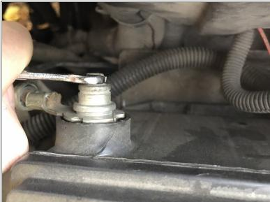
Using an 8mm wrench, disconnect the negative battery terminal. This is the one on the right (closest to the engine).
