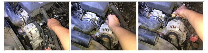
Remove the black wire from the back of the alternator using a 10mm socket and disconnect the voltage sensor. For the Voltage sensor, depress the tab towards the base of the sensor and pull outwards.
