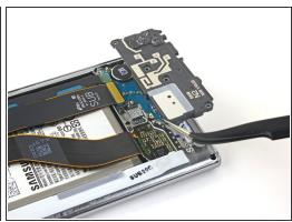
Use a pair of tweezers to remove the loudspeaker.
