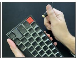
♠ Do not disassemble keyboard if it is connected to a power source.
