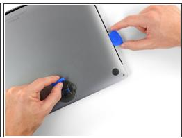
Repeat the previous step on the other side, using an opening pick to to release the second clip.
