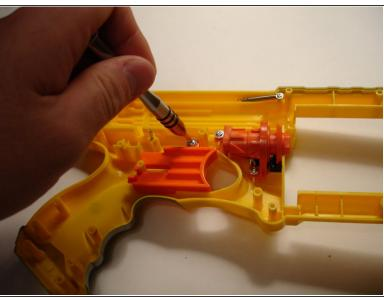
The trigger is held in place by a sole Phillips screw. It also has a small spring for that authentic handgun "springy" feeling...
