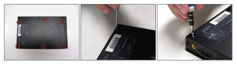
• After all of the feet have been removed, Use a Phillips #1 screwdriver to remove the six 4.0mm screws from the base of the PS2.
