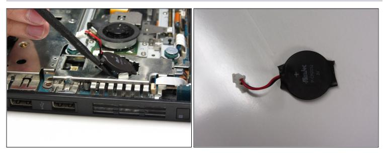
• Gently lift the battery up from the battery compartment using a spudger.
