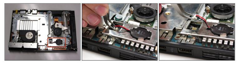
• Identify the clock battery, then use tweezers to disconnect the connector from the motherboard.
