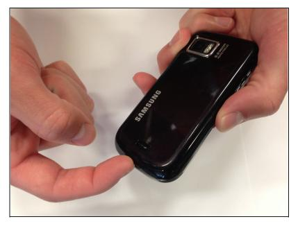
• To remove the phone's back cover, slide your fingernail into the slit at the bottom of your phone.
