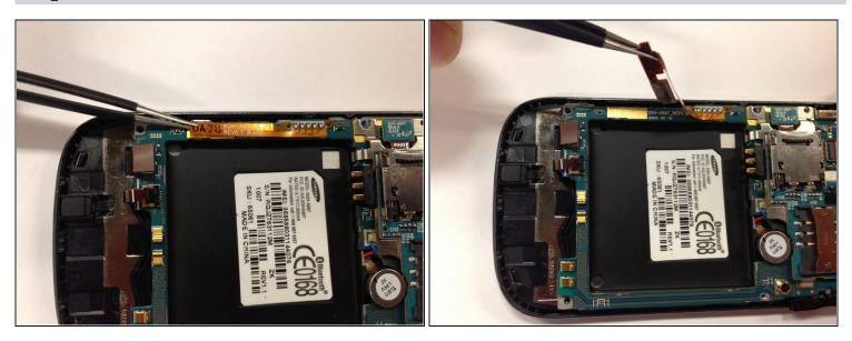
• Use the tweezers to unclip the orange ribbon cable from the left side of the phone.
