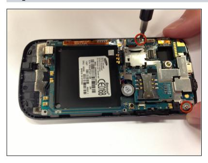
Using a Phillips #00 screwdriver, remove the two 3.8mm screws.
