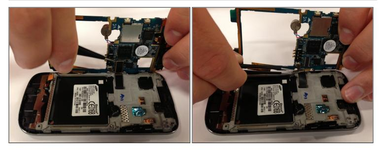
⚠ DO NOT remove the motherboard completely. One more clip on the motherboard's backside needs to be removed.
