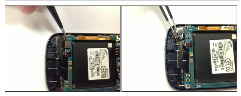
• On the right from the lever, use the tweezers to unclip the black connector.
