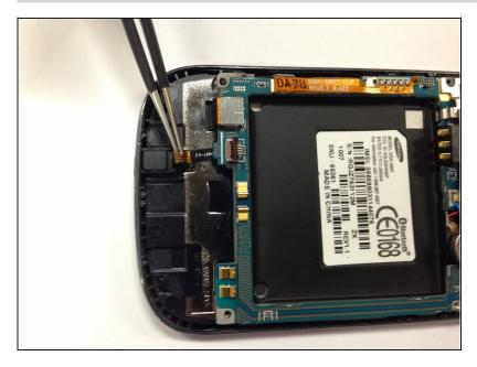
• Remove the ZIF cable by carefully using the tweezers to pull the cable straight out.
