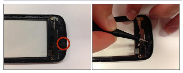
• Find the rubber microphone backing on the bottom of the back of the front cover as shown in the picture. Use <u>tweezers</u> to pluck the microphone from the casing.
