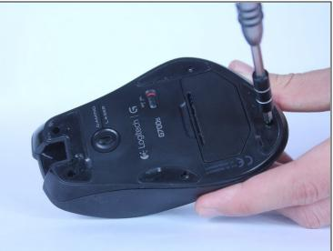
• Remove the five 5.5mm Phillips #00 screws found underneath the mouse feet.
