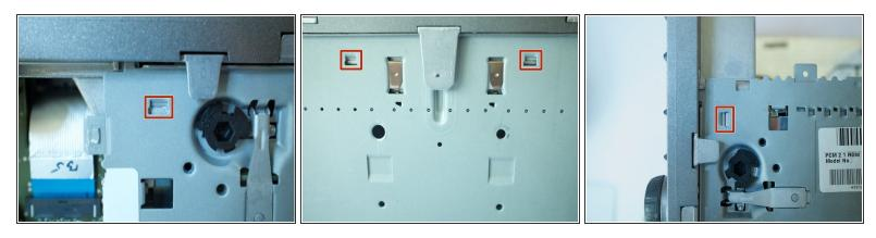
• This is the most difficult step in the process. Firstly, identify the four tab retainers holding the facia to the chassis. The three photos show them all.
