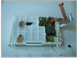
The first photo shows the location of the screen carrier clips. Once these are released with a spudger, the screen carrier can be released, the small grey ribbon connector can be gently pushed out the way when this is done.
