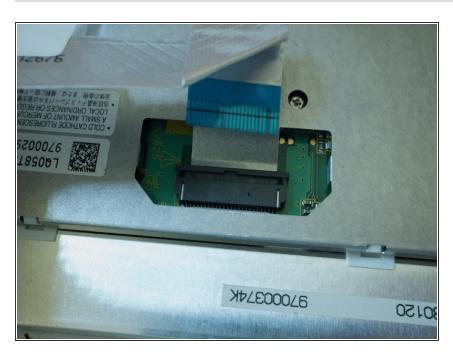
Disconnect the ribbon cable using the same technique that was done at the other end, where it connects to the motherboard.
