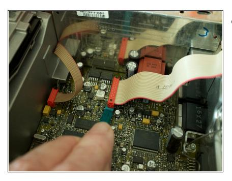
Use a plastic spudger to disconnect the PC ribbon cable joining the CD player to the motherboard and place the CD unit safely to one side.
