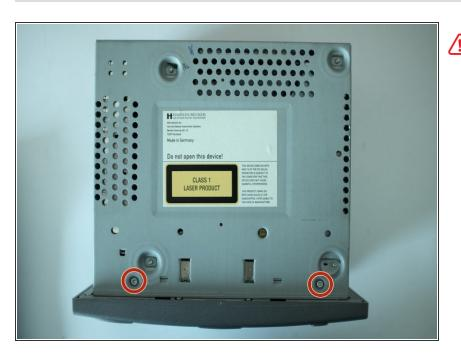
As the top of the unit says: the PCM should not be opened. Remove the two Torx T9 machine screws
