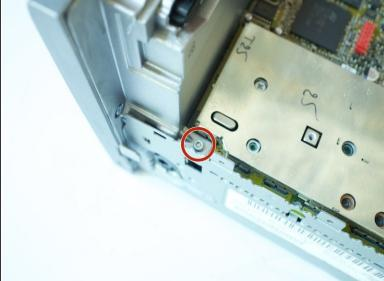
Remove the two Torx T9 machine screws that attach the front facia to the chassis. There is one screw either side as shown in the photos.
