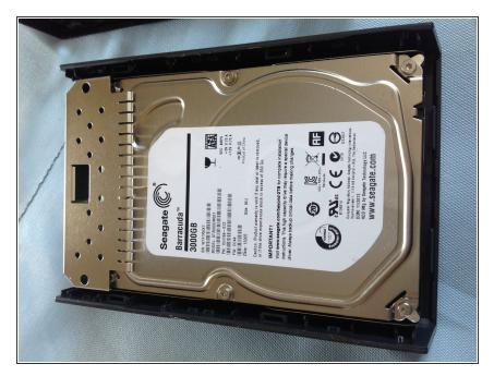
Gently pull the sides slightly and the drive will lift out
