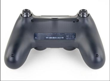
• Use a Phillips screwdriver to remove the four 6.4 mm-long screws from the rear panel.
