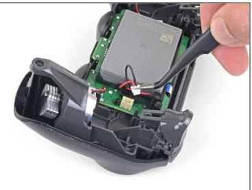
• Use a pair of <u>tweezers</u> to pull the battery's power connector straight up from the motherboard.
