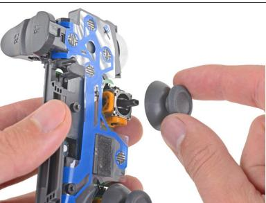
Pull the right joystick cover straight off the joystick module to remove it.
