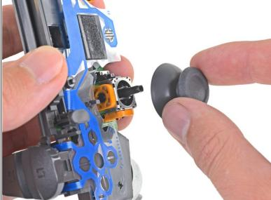
Pull the left joystick cover straight off the joystick module to remove it.
