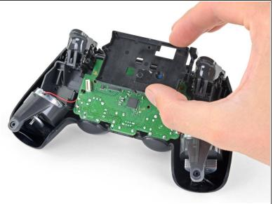
Remove the battery bracket.
