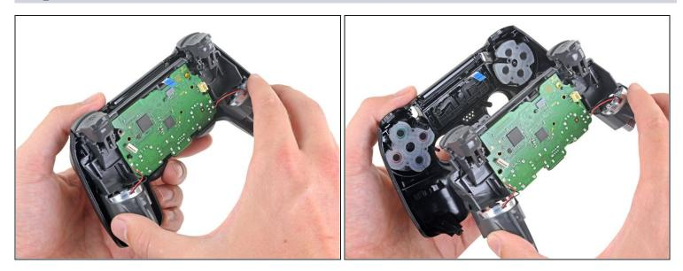
• Separate the motherboard and midframe assembly from the front panel.
