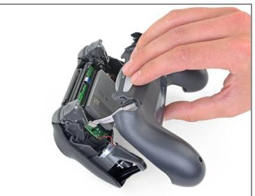
• Lift the rear panel directly away from the controller.
