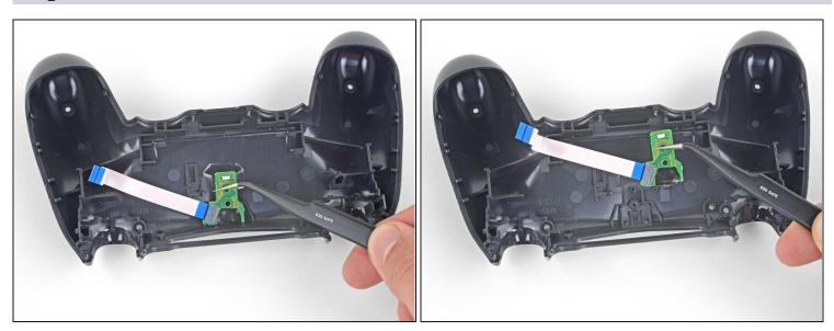
• Use your fingers or a pair of <u>tweezers</u> to remove the charging assembly from the rear panel.
