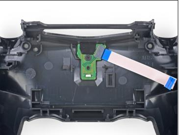
Use a Phillips screwdriver to remove the 4.4 mm-long screw from the charging assembly.
