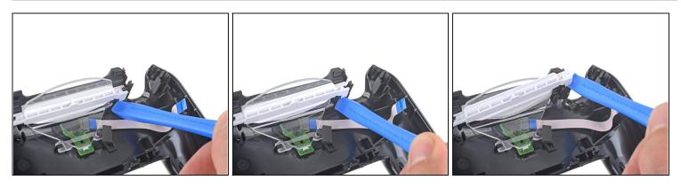
• Use an opening tool or spudger to separate the white plastic bar from the rear panel.
