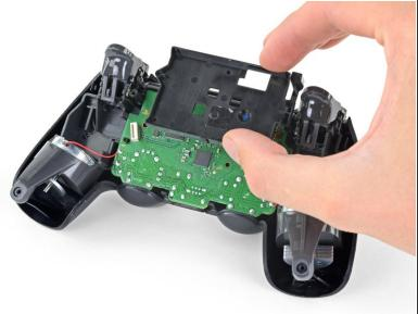
Remove the battery bracket.
