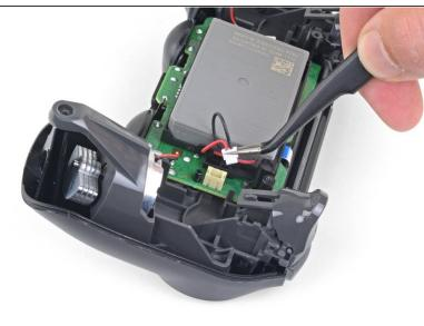
Use a pair of tweezers to pull the battery's power connector straight up from the motherboard.
