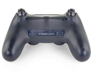
• Use a Phillips screwdriver to remove the four 6.4 mm-long screws from the rear panel.
