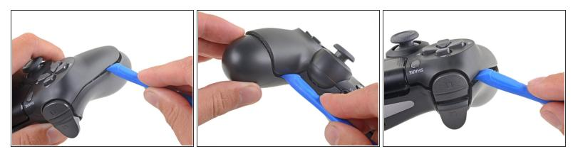
Use the opening tool to separate the panels by releasing the plastic clips around the perimeter of the controller.
