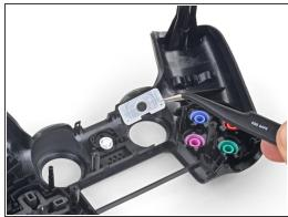
Use your fingers or a pair of tweezers to remove the three silicone conductive rubber pads from the controller buttons.
