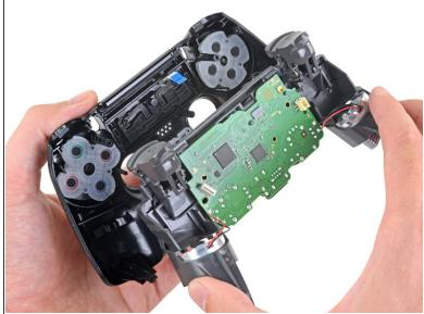
Separate the motherboard and midframe assembly from the front panel.
