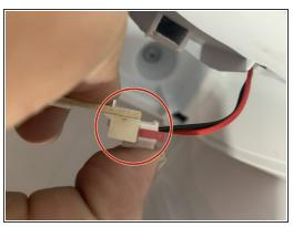
Disconnect the damaged light from the connection.
