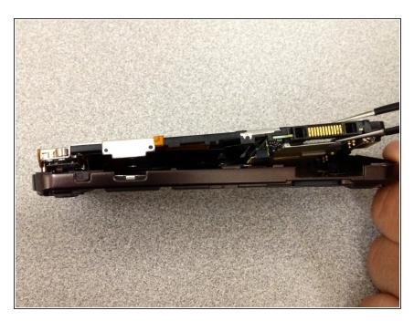
With a tweezer, pry off the back metal plate.
