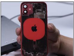
• Put the back glass of iPhone 12 under the focus positioning probe of the laser marking machine. After positioning, mark the back glass area except for the camera and wireless charging area. We haven't marked the wireless charging area to avoid damage.
