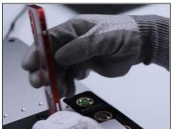
We should remove the wireless charging coil and then mark. The magnet array and shield can be easily removed after marking.
