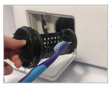
Using a toothbrush or damp washcloth, gently clean the inside and outside of the filter to remove leftover debris.
