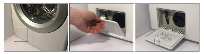
• Open the panel that is located at the bottom left of the washing machine.
