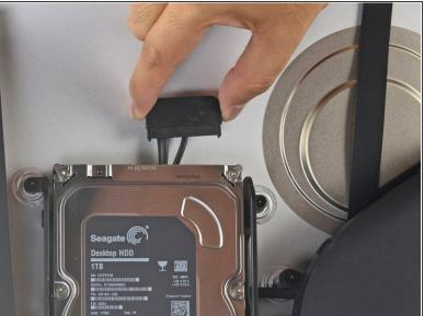
Pull straight up on the SATA combo cable to disconnect it from the drive.
