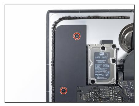
Use a T10 driver to remove the two 10 mm screws securing the left speaker.
