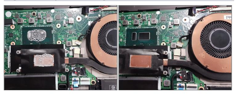
• Clean the old thermal paste both from the cooler and the CPU. It is best to use isopropyl alcohol and cotton swabs or paper towel, but be careful not to go too hard on the CPU.
