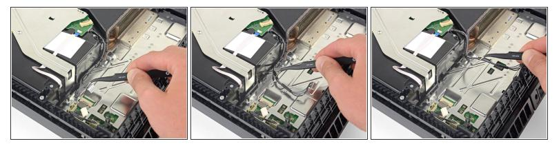
• Use your fingers or a pair of tweezers to remove the optical drive cable from the cable guides that hold it in place.
