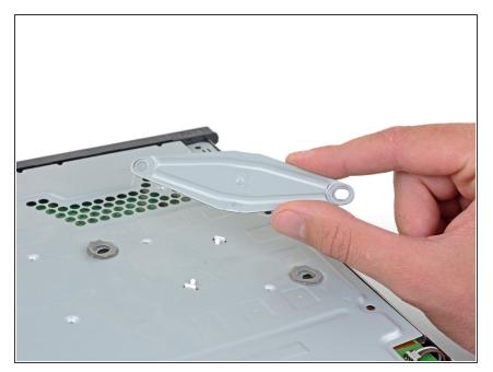
• Remove the pressure plate.
