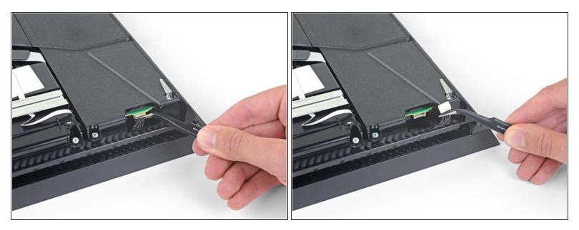
Use a pair of tweezers to pull the power supply cable straight out and disconnect the power supply unit from the motherboard.
