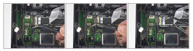
Use a pair of tweezers or your fingers to grab the antenna cable and move it out from the cable guides.
