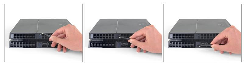
Use tweezers to remove the two stickers in the center of the back of the PS4 exposing two case screws.
