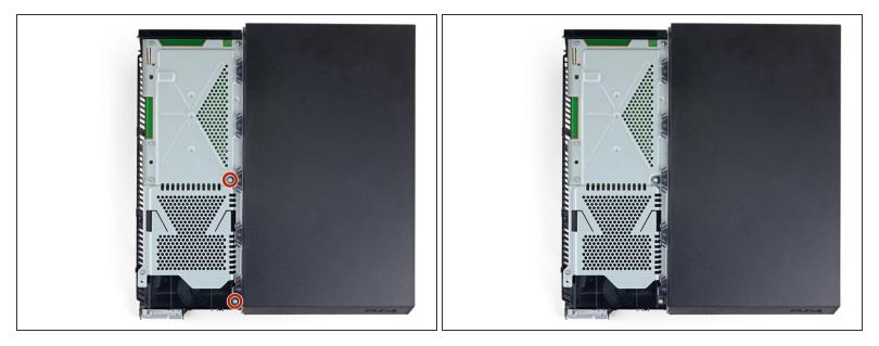
• Remove the two 9.7 mm Torx screws securing the upper case.
