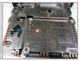
• Locate the six 1.6mm screws that mount the metal plate to the motherboard.
