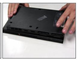
• Once all of the screws have been removed, pry apart the plastic covers. Start by lifting the side containing the power cable and Ethernet port. Then, lift the opposite side to fully separate the two sides.
