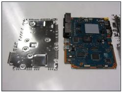
• Gently lift the metal plates from both the top and bottom of the motherboard.
