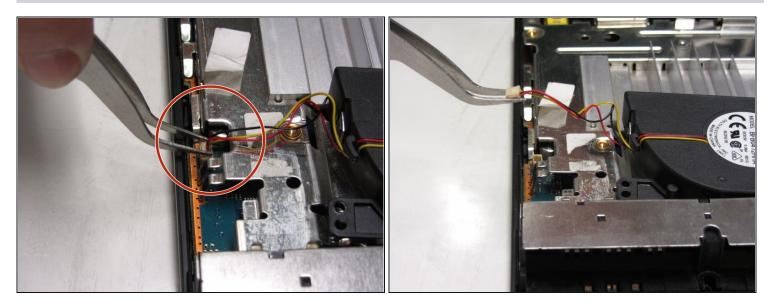
• Detach the terminal (white covering) to the red and yellow cords from the motherboard to the fan with the use of tweezers.
