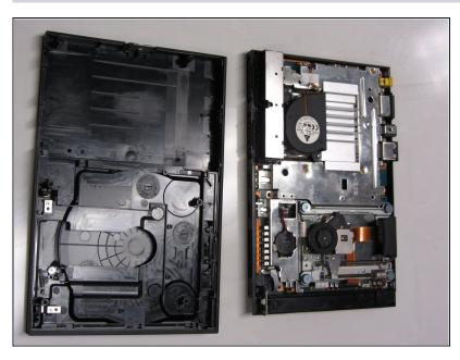
If done correctly, you should have a fully detached plastic backing, revealing the electronic components of the PlayStation 2.
