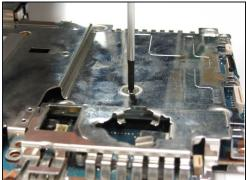
• Unscrew all six 1.6mm screws that mount the metal plate to the motherboard.
