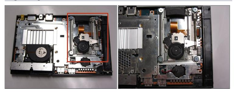
• Locate the optical drive on the motherboard.
