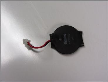
• Gently lift the battery up from the battery compartment using a spudger.
