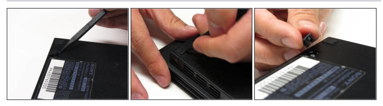
• Remove the five visible feet from the bottom of the device using a spudger.
