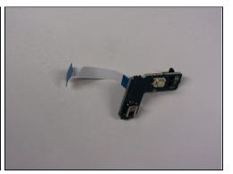
• Locate the IR sensor on the motherboard. Then, use tweezers to gently detach the blue/white ribbon that attaches the IR sensor to the motherboard.
