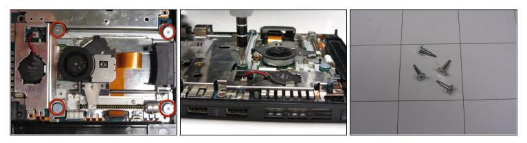
• Unscrew the four 4.0mm screws that mount the optical drive to the motherboard.
