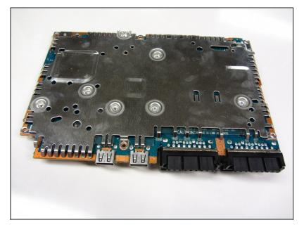
Locate the metal plate that is attached to the back of the motherboard.
