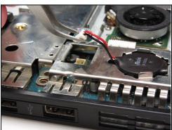
• Identify the clock battery, then use tweezers to disconnect the connector from the motherboard.
