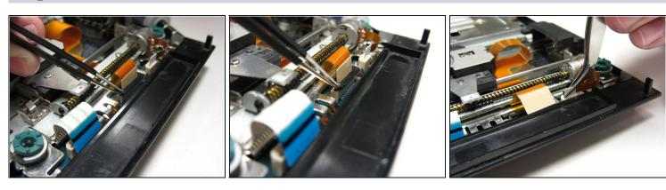
• Using tweezers, gently detach all three ribbons from the motherboard terminal. Unlock the middle orange ribbon to lift the black tab up on either side.
