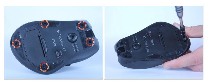
Remove the five 5.5mm Phillips #00 screws found underneath the mouse feet.
