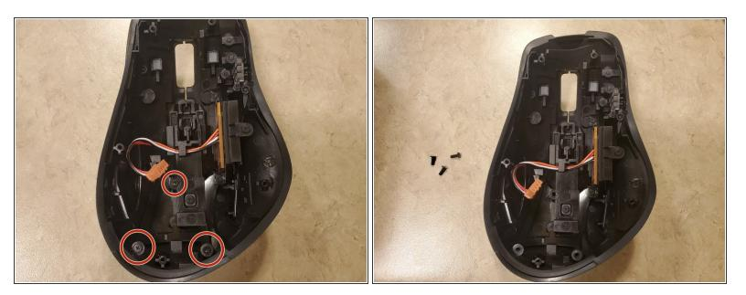
• Remove the three Philips head screws holding the left and right button clicker in place
