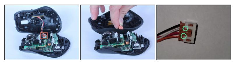
• Pull the top of the mouse off of the bottom half.
