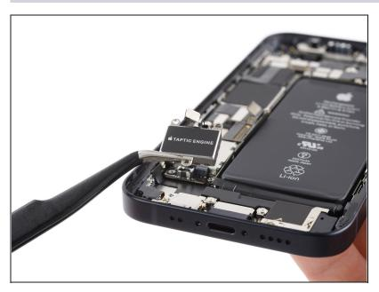
• Use a pair of tweezers to remove the Taptic engine.
