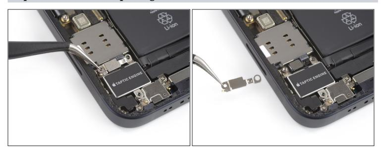
• Use a pair of tweezers to remove the Taptic engine connector cover bracket.
