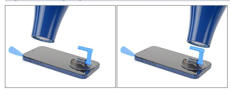
• Use a hair dryer to heat the right edge of the iPhone (the edge with the power button) for 90 seconds or until the screen is slightly too hot to touch.
