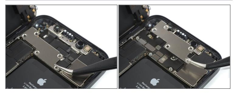
• Use a pair of tweezers to remove the front sensor assembly bracket.
