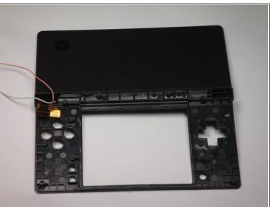
• Flip the case open, and push the lower screen assembly out of the frame.
