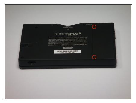
Loosen the two screws on the battery panel. Then lift the panel up to remove it.
