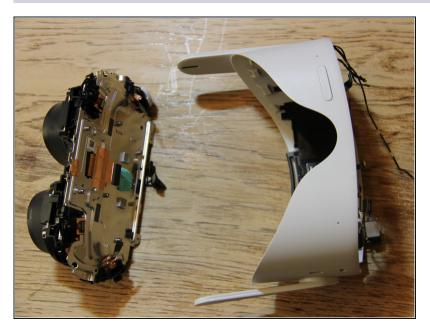
• The midframe is removed giving access to the battery.
