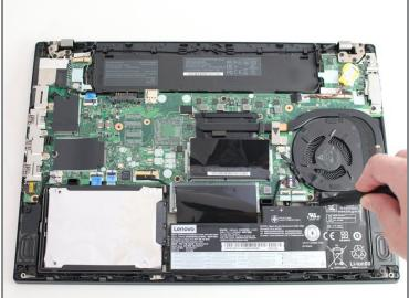
• Using the Phillips #1 screwdriver, remove the two 4.6 mm screws securing the internal battery to the frame.
