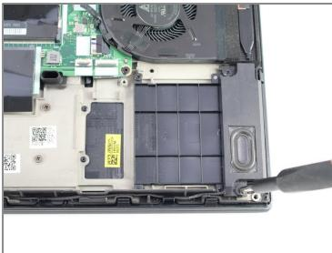
• Using the Phillips #1 screwdriver, remove two 4.8 mm screws from the right speaker.
