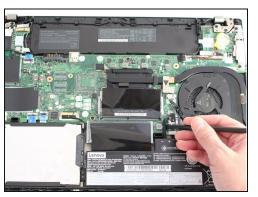
• Use the spudger to slide the battery socket connector parallel to the motherboard and out of its socket on the motherboard.
