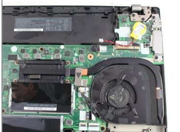
• Using an IC extractor or black nylon spudger, unplug the connector from the socket on the motherboard.
