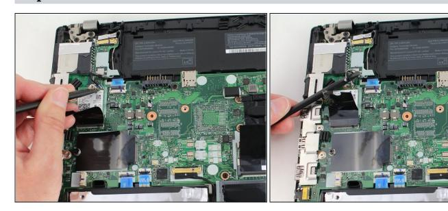
• Insert the point of a spudger under one of the antenna cables close to the connector. Pry straight up to disconnect the cable off of the Wi-Fi card.
