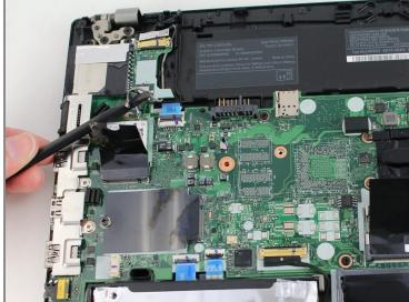
• Insert the point of a spudger under one of the antenna cables close to the connector. Pry straight up to disconnect the cable off of the Wi-Fi card.
