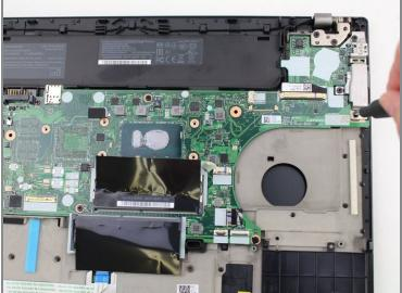
• Using the Phillips #1 screwdriver, remove three 4.6 mm screws from the I/O bracket.
