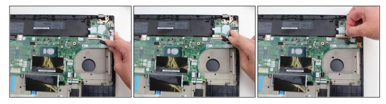
• Use the tip of a spudger or an opening tool, to flip up the small, hinged locking flap on the camera cable connector to remove the cable from the motherboard.
