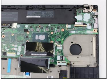
• Lift the I/O bracket off the motherboard.
