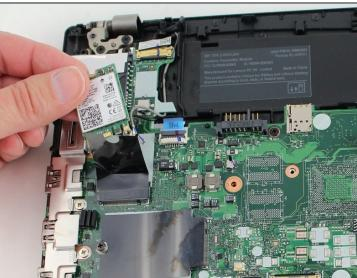
• Slide the Wi-Fi card out from the slot to remove it from the board.
