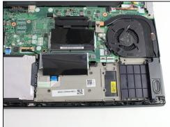
• Using the black nylon spudger, wedge the battery up from the case and lift it out.
