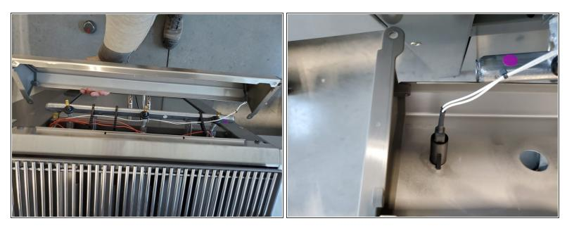
Disconnect the cables from the ignitor.
